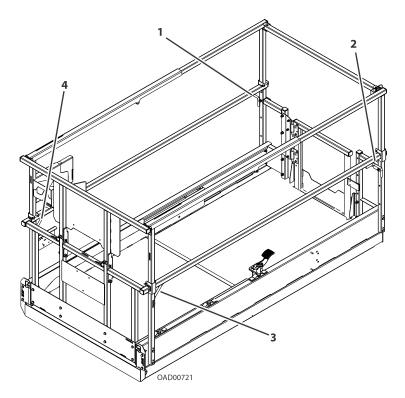
**Figure 3. Lanyard Attach Points**
