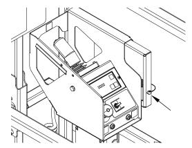
To prevent unauthorized removal, the platform control station can be secured to its mount by replacing the lock pin located on its mounting tab with a keyed or combination lock.
