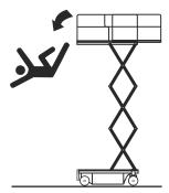
Keep both feet firmly positioned on the platform floor at all times. Never position ladders, boxes, steps, planks, or similar items on unit to provide additional reach for any purpose.
