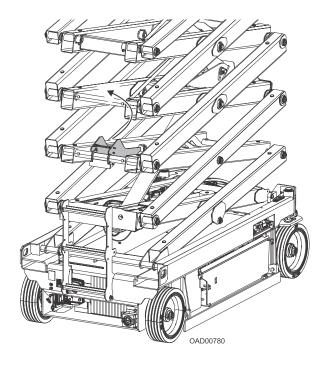
Figure 12. Prop Disengaged
