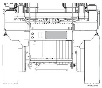
Figure 10. 2632 Serial Number Plate
