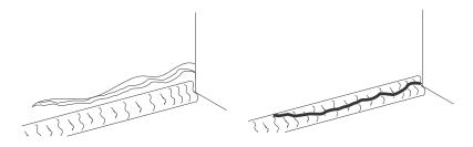
Figure 1. Parent Metal Crack
