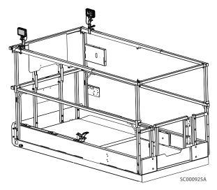
The Platform Worklights accessory consists of two 12V lights mounted to the platform railings.
